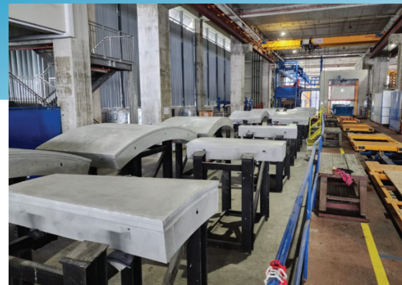
Above: Construction of hydraulic tunnel linking Tuas Water Reclamation Plant and Jurong Island. Using OPC and steel reinforcement bars would have generated 736 kg of CO 2 per m 3 of concrete. The adopted solution using fly ash cement, OPC, silica fume and steel fibres generated only 328 kg of CO 2 per m 3 of concrete, more than halving the carbon emissions.
